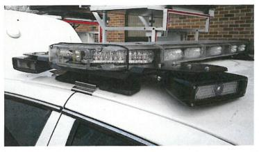
Project Description: The ALPR unit will scan/read license plates on vehicles that pass the device. The Brentwood Police Department would utilize this device to scan for expired registrations, warrant suspects, and amber alerts. The scanner automatically checks the license against a database for any violation.
